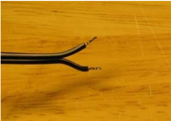
Finished wire ends.
